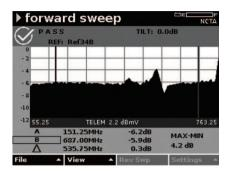
Forward sweep on the DSAM-6000 uses a unique referencing method to accurately reveal any problems in the system without interfering with any of the analog or digital carriers.
