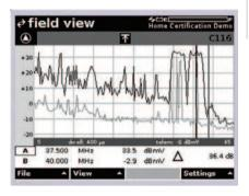
The optional Field View capability greatly improves the success rate and efficiency in locating ingress on the return path. Field technicians can view the return spectrum as received by the JDSU PathTrak Return Path Monitoring System. Both the remote spectrum and the local spectrum view can be compared on the tech's meter.
