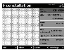
A Constellation graph shows impairments on the network with patterns in the display. By identifying the pattern technicians can figure out what is the probable cause of the impairment.
