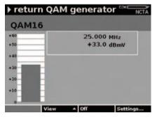
The Return QAM Generator eanables operators to test and prove upstream network performance.
